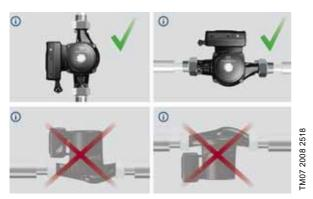
Fig. 34 Control box positions
