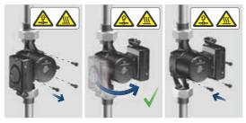
Fig. 38 Changing the control box position
