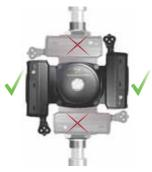
Fig. 36 Allowed control box positions
