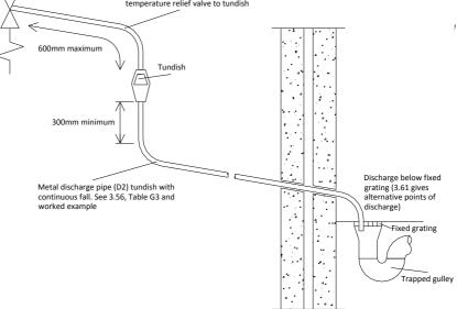
Figure G3: Typical discharge pipe arrangement
